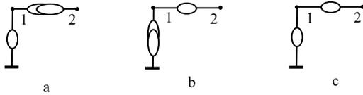
Fig. 8. Equivalent grounded trees with VM and/or nullators.
