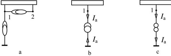
Fig. 6. Trees with VM, connected to ground node (a); single CM (b) and norator (c), connected to ground.
