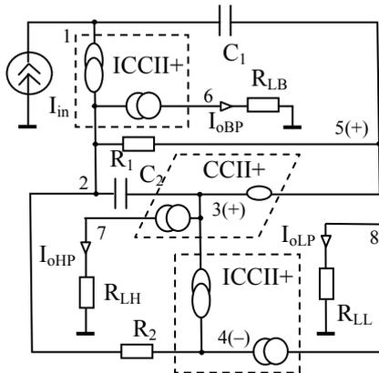
Fig. 10. The first equivalent circuit (for the circuit on Fig. 9) based on two ICCII+ and a CCII+, in which one of VM is replaced by nullator.
