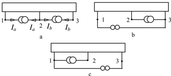
Fig. 5. Connection of trees with CM and norator elements to some circuit: original CM tree (a), equivalent CM and norator trees (b) and (c).
