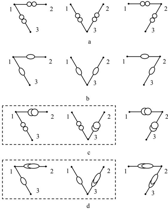
Fig. 2. Equivalent trees of pathological elements: nullators (a), norators (b), voltage mirrors and nullators (c), current mirrors and norators (d).
