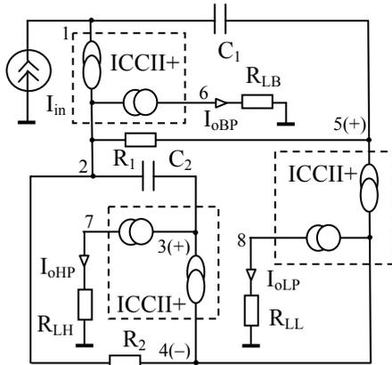
Fig. 9. Universal filter circuit based on three ICCII+.
