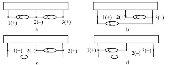
Fig. 3. Connection of the trees of VM and nullator to some circuit: original tree of VM elements (a), non-equivalent tree of VM elements (b), equivalent trees of VM and nullator (c) and (d).
