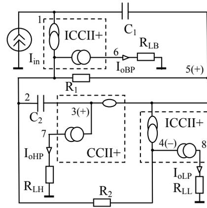
Fig. 11. The second equivalent circuit (for the circuit on Fig. 9) based on two ICCII+ and a CCII+, in which one of VM is replaced by nullator.
