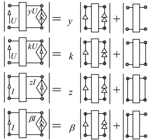
Figure 2: Extraction of the element parameters.
