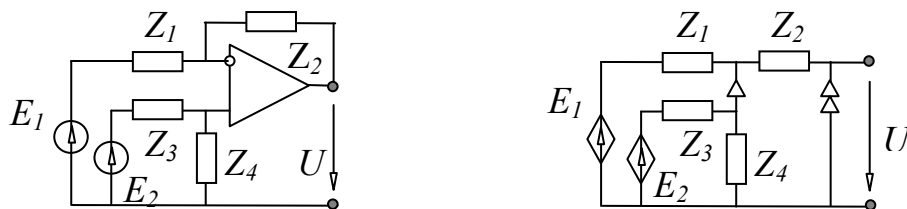
Fig.10. Differential amplifier (a), nullor based equivalent circuit (b).
